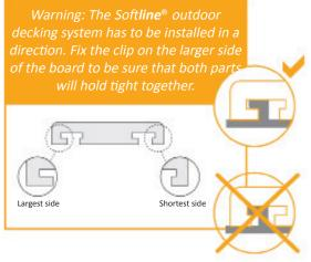
• Fit the planks in the clips, the wide side of the planks entering the clip (see diagram below), assemble the planks end in one another through special tongue already placed. The space of 6.5 mm between the planks will automatically be respected by the spacers, this space is intended to guarantee a good ventilation of the decking. The following plank must be placed completely into the clip in order to be insert longitudinally in the head of the plank (see drawing).
