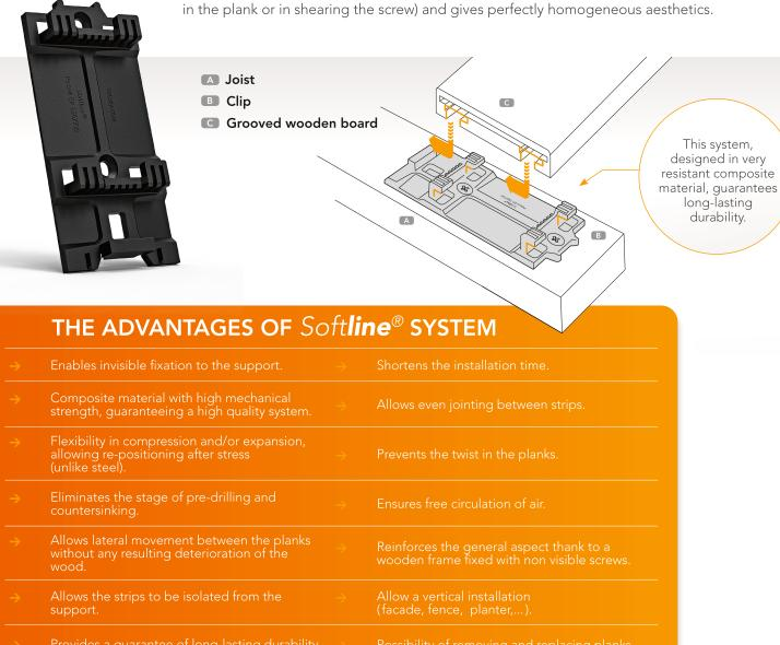
The Softline® fixation system allows free circulation of air and movement between the planks without any resulting deterioration of the wood.
